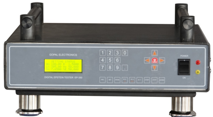
High Precision Epstein Tester 25Hz TO 450Hz Source
